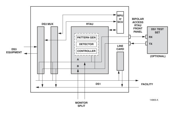
Figure 570-6. RTAU Test Configuration Block Diagram
